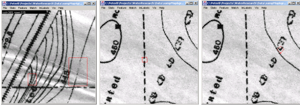
Figure 8: Examples of contour gaps and parallel lines in proximity (left), dashed line (middle) and touching symbol (right) delineated with a rectangular.
