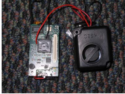
Figure 13: MICA2 Mote with powerful speaker.
