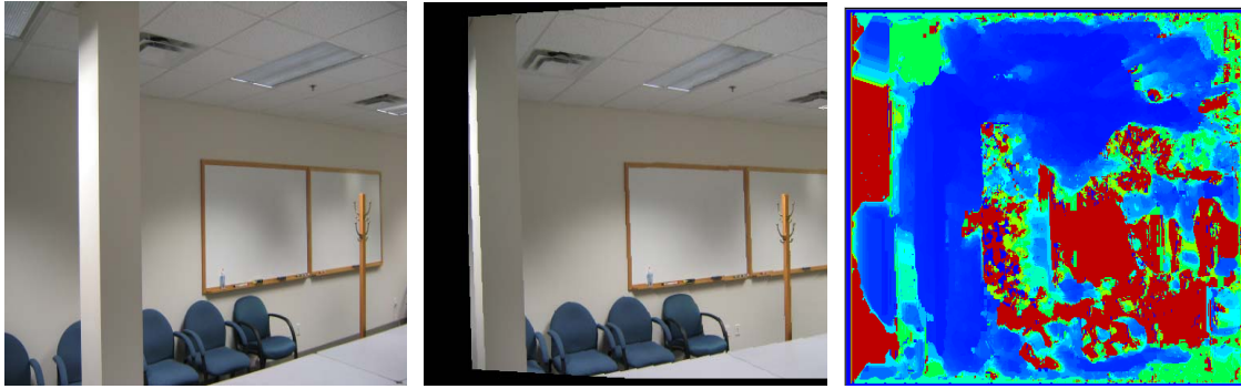
Figure 10: Measured Laboratory Images (Room without Added Texture). Left and Middle – The input [rectified] stereo images, Right – Computed depth map (black – invalid, cool – close to viewer, warm - far from viewer)
