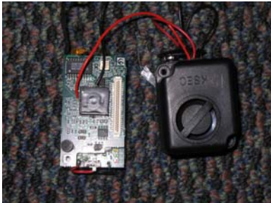
Figure 23: MICA2 sensor with a powerful sounder that was borrowed from the CS Department, UIUC.
