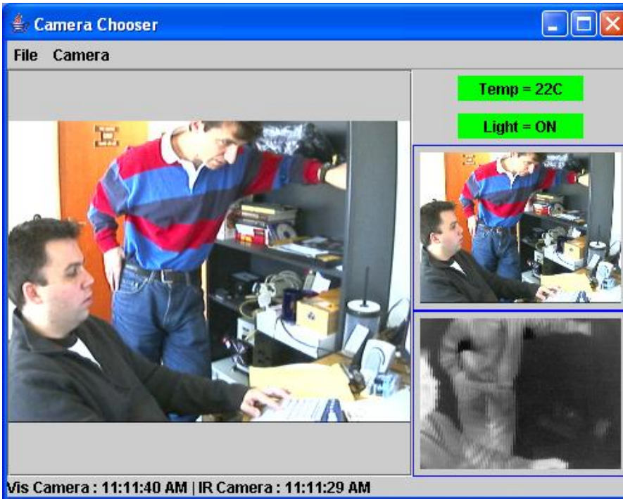
Figure 28: Proactive camera control. Depending on the temperature and light readings from a wireless network of motes, either a visible spectrum video or a thermal infrared spectrum video is sent to a hazard monitoring station.
