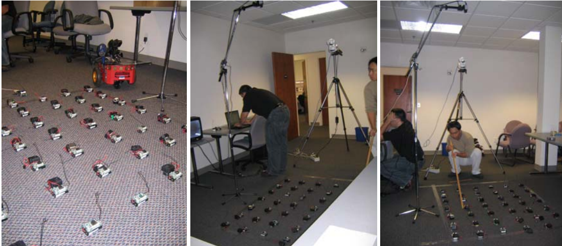
Figure 24: Experimental calibration setup with MICA2 sensors on the floor, thermal IR camera located close to the ceiling and pointing straight down, and visible spectrum camera located close to the door and providing these setup pictures. A robot with a hair dryer was used to simulate temperature changes (see the left picture).
