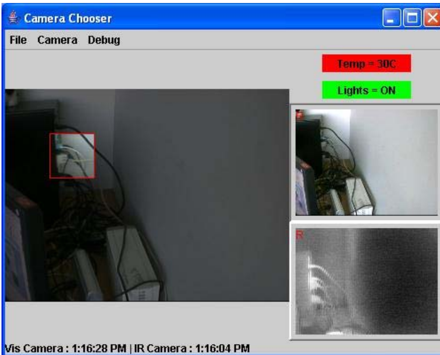
Figure 29: Illustration of hazard alert by automated region selection and image enhancement. Note how the system uses the RGB camera when the office light is on, and combines the information about white (hot) regions from the thermal IR camera to highlight the RGB region of interest (the hazard region).
