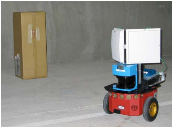
Figure 2. This figure, adopted from Philipose et. al. [7], illustrates the experimental setup and learning a probabilistic sensor model for the RFID antenna.
