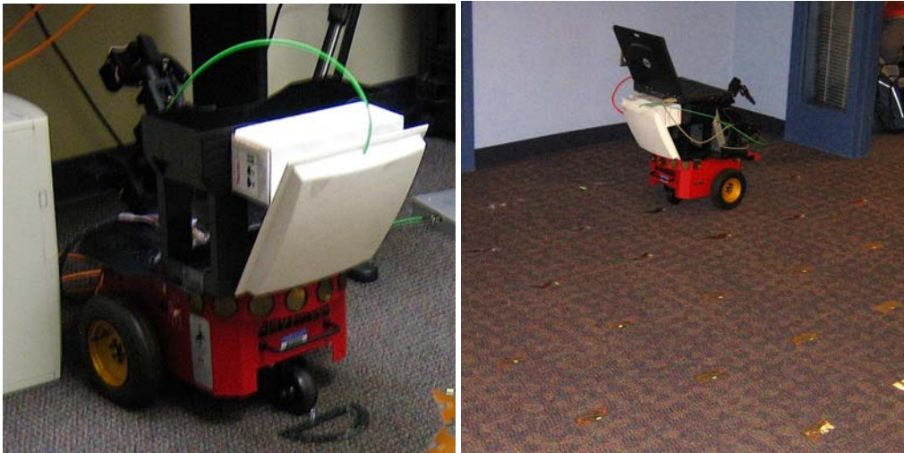
Figure 4. Experimental setup. The Alien Reader was mounted on the platform of a robot (left). The RFID tags were placed on the floor in a regular grid pattern (right).
