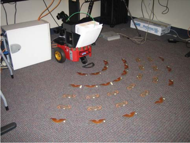
Figure 3. Left: documentation of setup used to build the sensor model. Right: Image showing nominal detection range when Tags are distributed on the floor and the Reader is mounted on the robot and tilted forward 60 degrees. The 4th "row" has a radius of roughly 90 cm.
