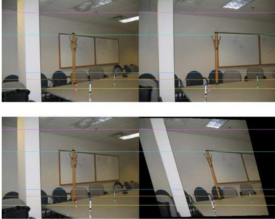
Figure 2.4: Stereo Rectification Example
