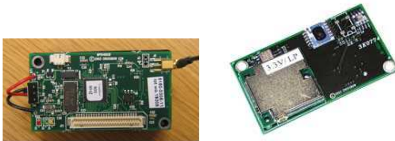
Figure 1.2: Crossbow MPR400 MICA2 Sensor and Crossbow MTS420 Sensor Board
