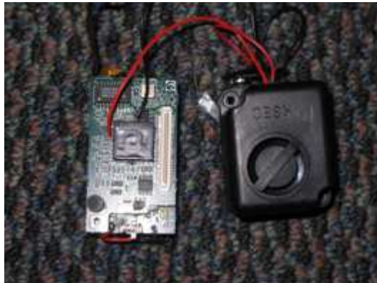
Figure 3.6: MICA2 Mote with Loud Speaker
