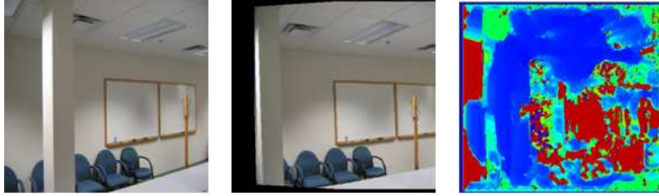
Figure 2.9: Measured Laboratory Images (Room without Added Texture). Left and Middle: The input [rectified] stereo images, Right: Computed depth map (black: invalid, cool: close to viewer, warm: far from viewer)
