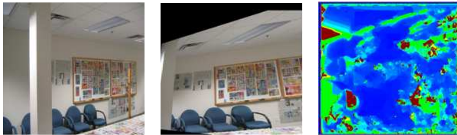
Figure 2.10: Measured Laboratory Images (Room with Added Texture). Left and Middle: The input [rectified] stereo images, Right: Computed depth map (black: invalid, cool: close to viewer, warm: far from viewer)
